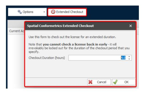
Press **Extended Checkout** button and in its window type the amount of hours required. This will lock the license to your machine (online and offline) for the duration of the checkout.
